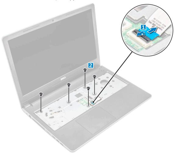
Remove the screws that secure the base cover to the computer
