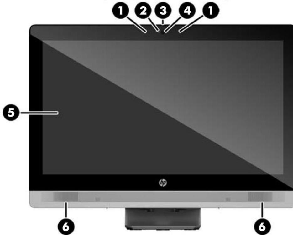
1. Dual microphone array (with webcam)
