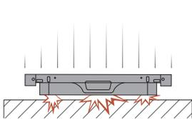
Be careful not to expose the product to vibrations or external shocks when it is lying flat on the floor.
