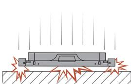
After removing the protective brackets, do not place the product on the floor with the LED facing down.
