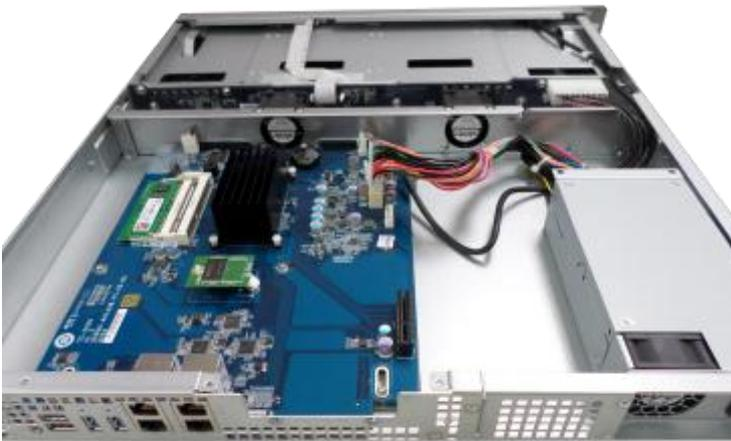
3. Slide the memory module to the slot at a 45-degree angle (approximately).
