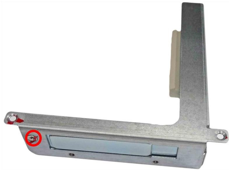
8. Insert the new network expansion card to the riser card module until it cannot go any further. Then fasten the screw.
