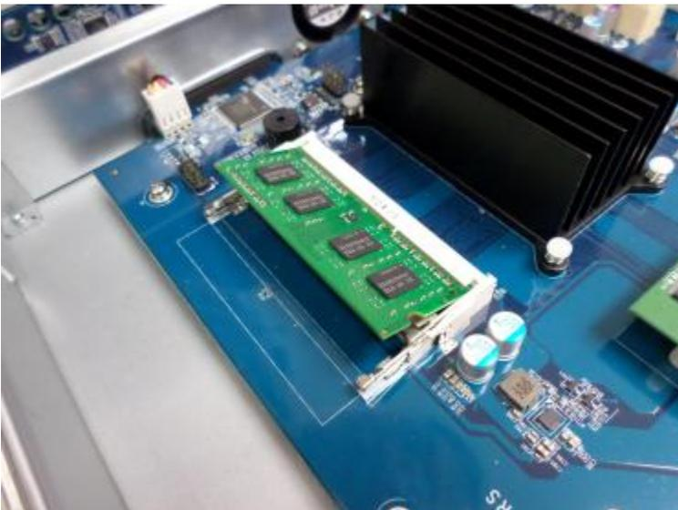
4. Press the memory module down. Make sure the memory module sits in properly with the clips in place.
