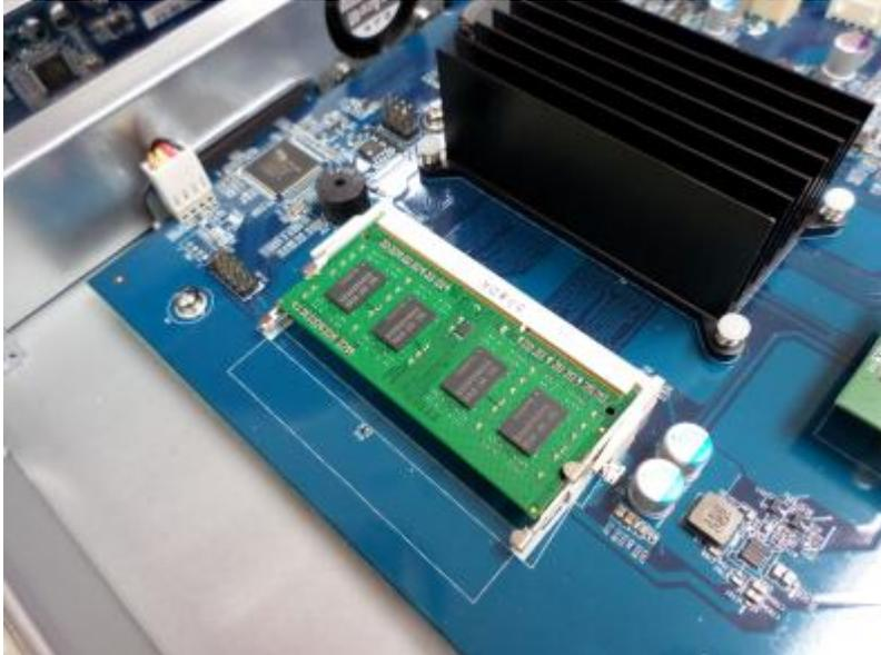
**Note: For TS-x53U & TS-451U models, always ensure that a memory module is installed in the primary slot (red box in the below figure,) or the system will fail to start.** When installing two memory modules, please ensure that they are the same size and ideally use the same type of RAM for both memory slots. The maximum supported memory is 8GB combined.
