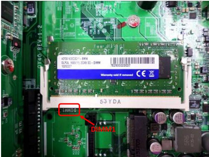
3. Slide the memory module to the slot at a 45-degree angle (approximately) and press the memory module down until it clips into place. Ensure the memory module sits properly with the clips in place.
