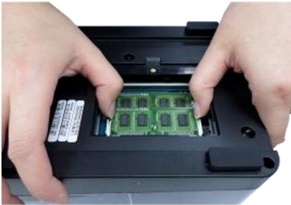
**Note: Always ensure that a memory module is installed in the Primary (red) slot. If not, then the system will fail to start.** When installing two memory modules, please ensure that they are the same size and ideally use the same type/model for both slots.
