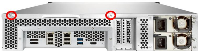
4. Hold the notch at the edge of the top cover. Remove the top cover in both hands.
