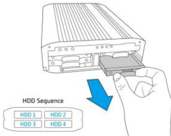
3. Attach the drive to the tray and secure the four screws in the back of the drive tray.
