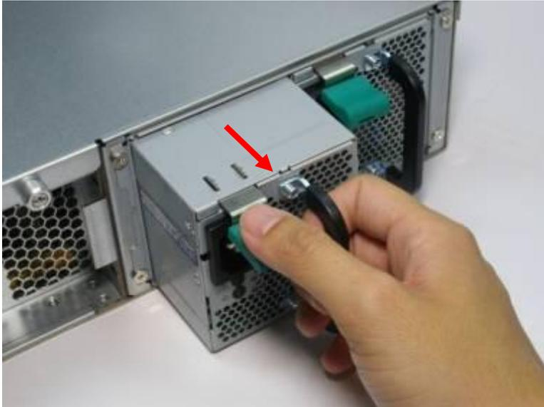
4. Plug in a new power supply to the NAS.
