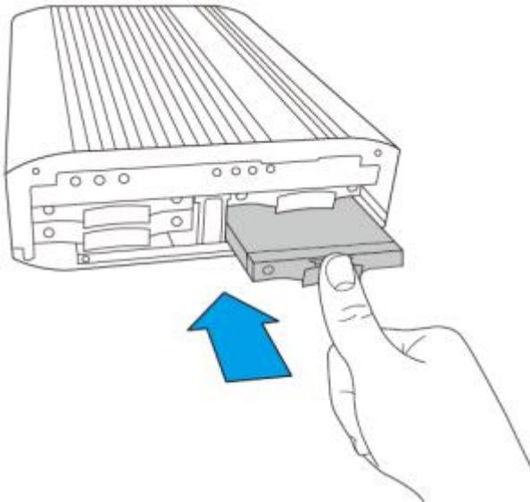
5. Repeat Step 2 to 4 to install the remaining drives. Please follow the HDD Sequence shown in Step 2 to do so.
