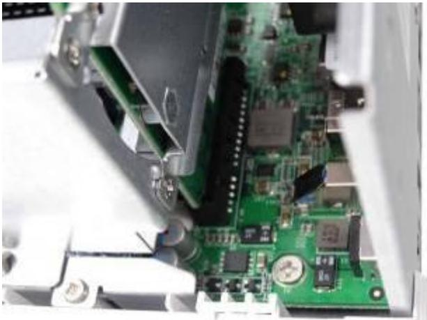
6. **Always ensure that a memory module is installed in the Primary slot (red). If not, then the system will fail to start.** When installing two memory modules, please ensure that they are the same size and ideally use the same type of RAM for both memory slots. The maximum supported memory is 8GB combined.
