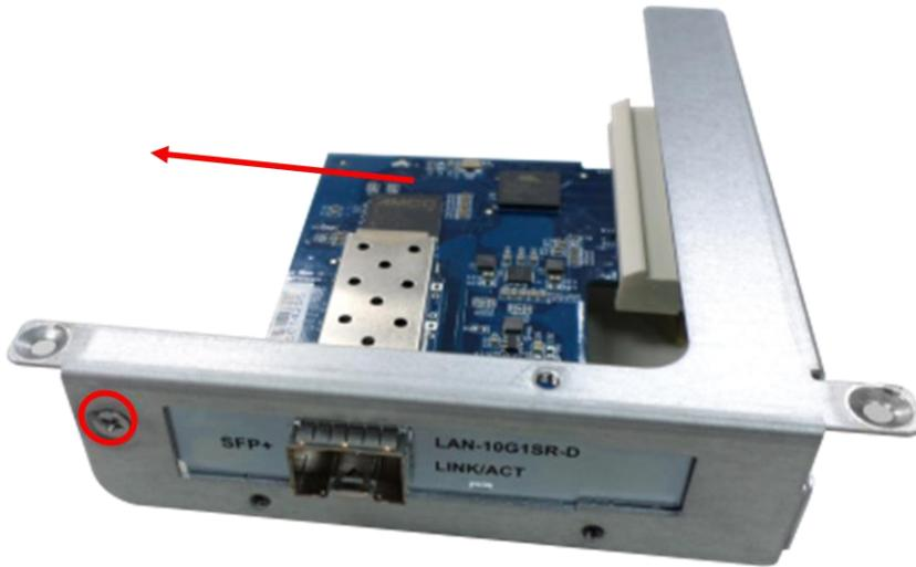
b. For TVS-471U, loose the screw and remove the bracket
