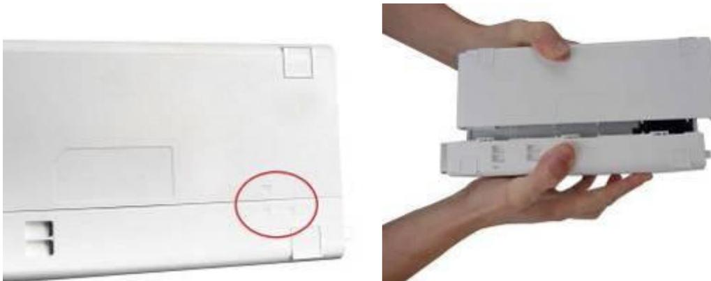
3. Remove the four inner screws (two on each side) of the hard drive cage.
