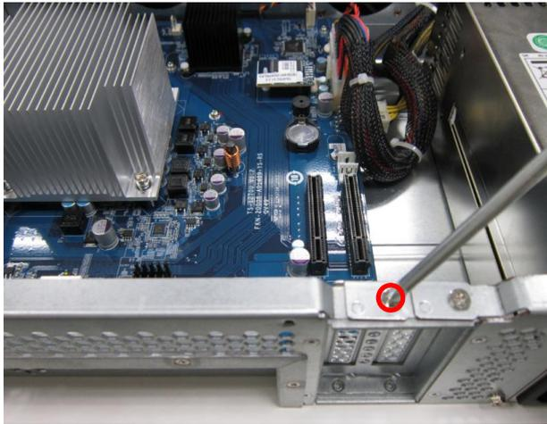
6. Grasp the edge of the expansion card. Align the notch on the gold edge of the card with the notch in the PCIe slot. Insert the network expansion card to the PCIe slot until it cannot go any further.
