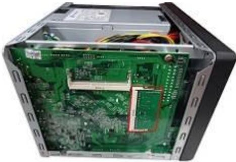
4. Grasp the edge of the memory module. Align the notch on the gold edge of the module with the notch in the memory slot. Slide the memory module to the slot at a 45-degree angle (approximately).
