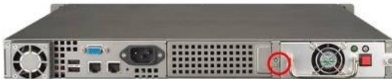
3. Insert the power supply unit and push it to the end.
