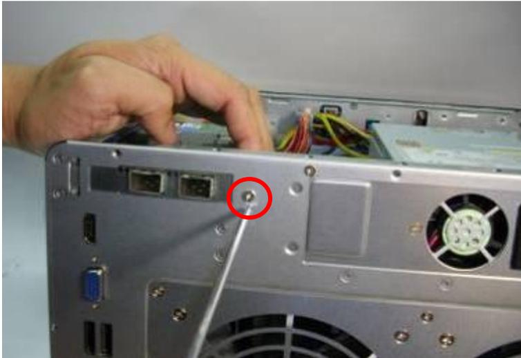
8. Close the case cover and fasten the screws. Connect the power adaptor and cables to the NAS.
