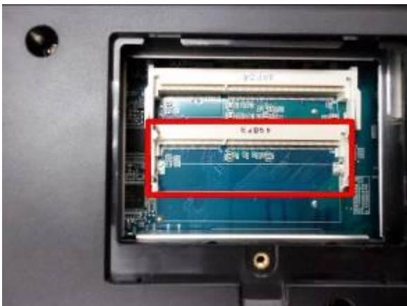
3. Slide the memory module to the slot at a 45-degree angle (approximately) and press
