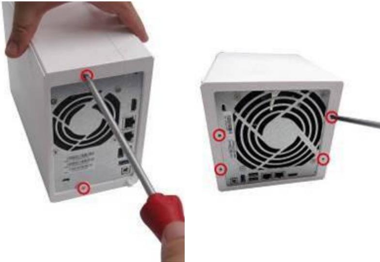
2. Gently remove the case cover of the NAS by sliding it apart (see the underside of the NAS for visual indicators of the NAS case being locked/unlocked)
