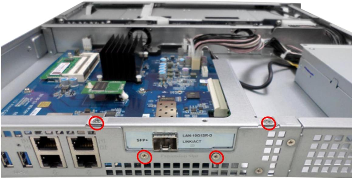
6. Grasp the metal edge of the riser card module. Remove the module gently.
