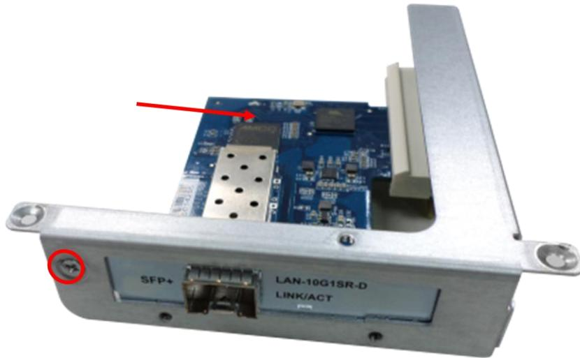
9. Align the notch on the gold edge of the riser card with the notch in the PCIe slot. Insert the riser card module to the PCIe slot until it cannot go any further.
