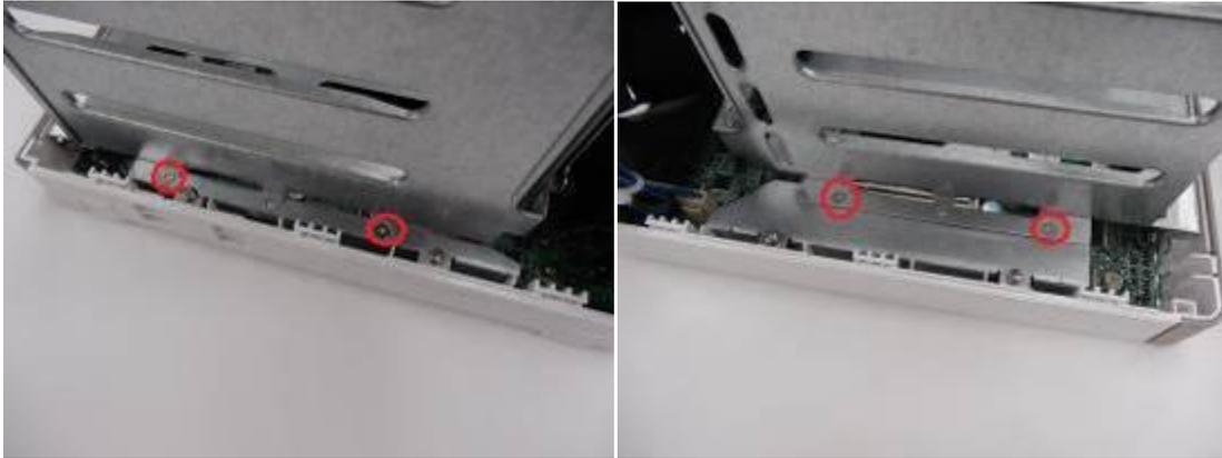
4. If it is a 4-bay NAS, you will also need to remove two screws on the top of the hard drive cage.
