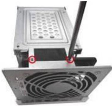
5. Gently remove the hard drive cage from the NAS by lifting it out of its slot.
