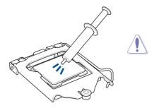
Apply the Thermal Interface Material to the CPU cooling system and CPU before you install the cooling system, if necessary.
