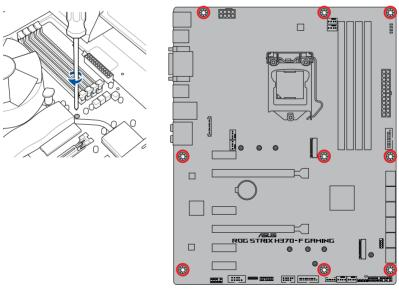
DO NOT overtighten the screws! Doing so can damage the motherboard.
