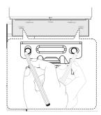
3. Remove the Wall bracket install guide.
