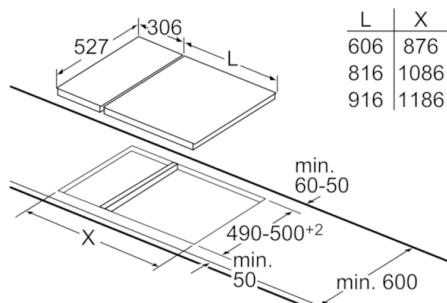
When installing a Domino unit right next to a hob, an assembly kit (HEZ394301) is required.
