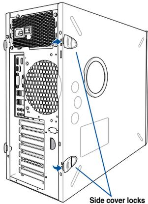
3. Slightly pull the side cover toward the rear just enough to detach it from the chassis.
