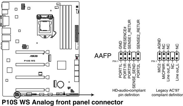
**P10S WS Analog front panel connector**
