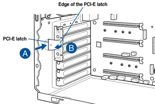
3. Remove the screw (A) that secures the metal bracket to the chassis then remove the metal bracket (B).
