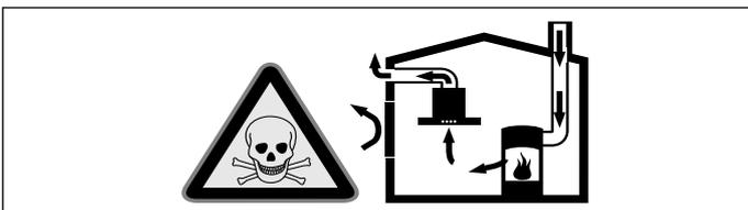
Non-room-sealed heating appliances (e.g. gas-, oil-, wood- or coal-burning heaters, continuous flow heaters or water heaters) draw in combustion air from the room in which they are installed and discharge the exhaust gases outdoors through an exhaust gas system (e.g. a chimney).
