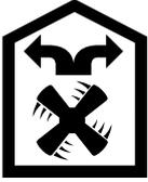
The air that is drawn in is cleaned by the grease filters and an activated carbon filter and conveyed back into the kitchen.
