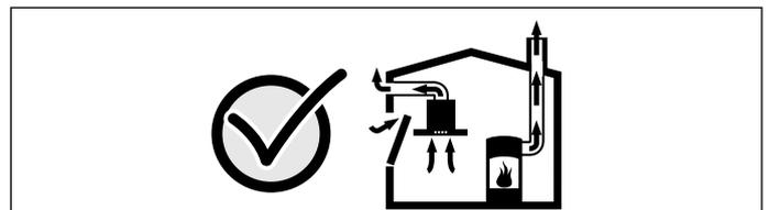
Always consult the heating engineer responsible. They will be able to assess the house's entire ventilation setup and suggest the most appropriate ventilation measures. Unrestricted operation is possible if the extractor hood is operated exclusively in air recirculation mode.
