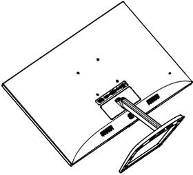
2. Use your fingers to loosen the screw located at the bottom of the base, and remove the base from the stand.
