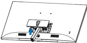
4. Use a screwdriver to remove the screws on the arm, and then detach the arm/stand from the monitor.
