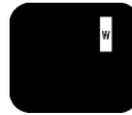
Three adjacent lit sub pixels (one white pixel)
