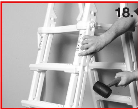
**18.** Lay ladder on its side, put a little liquid soap onto the square ends of the treads. Next place the tread connector onto the ends of the treads and strike hard with a rubber mallet to seat tread connector onto the treads. Flip ladder over and repeat for second tread connector.
