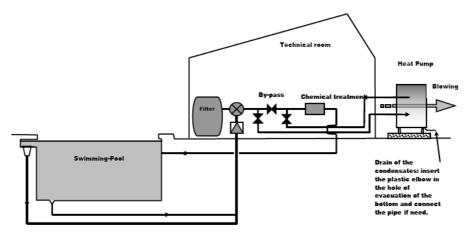
Figure 6: Typical hydraulic circuit part layout.
