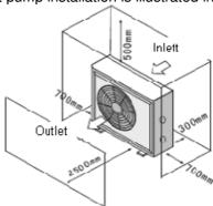
Figure 2: Clearance required for correct installation.
