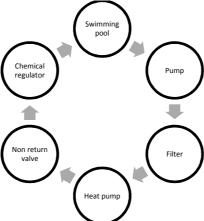
Figure 4: General hydraulic circuit layout.
