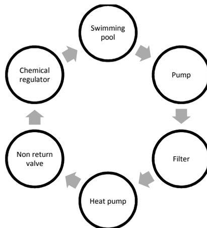
Figure 4: General hydraulic circuit layout.
