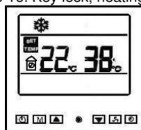
Figure 17: Key lock, cooling mode.
