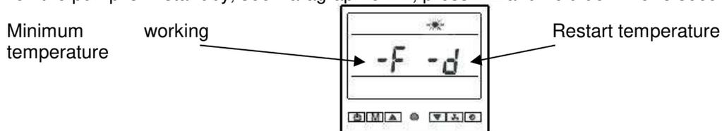
Figure 12: Minimum working temperature and restart temperature.
