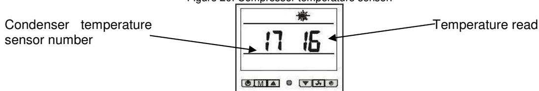
Figure 21: Condenser temperature sensor.
