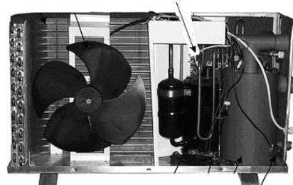
Figure 27: Compressor temperature sensor.
