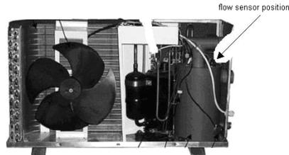
Figure 25: Flow sensor position.
