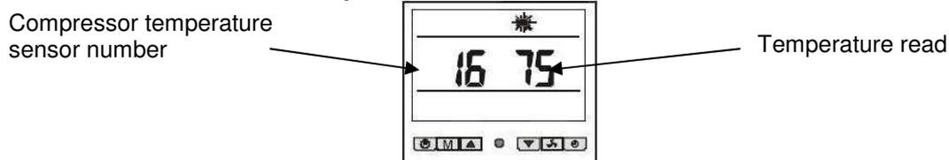
Figure 20: Compressor temperature sensor.
