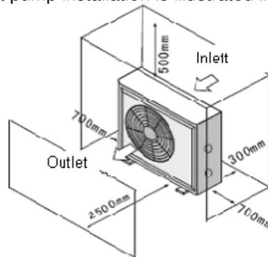
Figure 2: Clearance required for correct installation.
