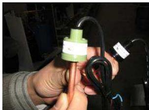
Figure 28: High pressure sensor.
