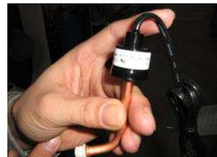
Figure 29: Low pressure sensor.
