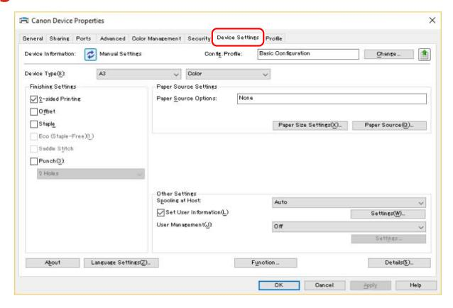
4 Check whether the configuration profile is suitable for the device you are using → if it does not match printer model, click [Change].
