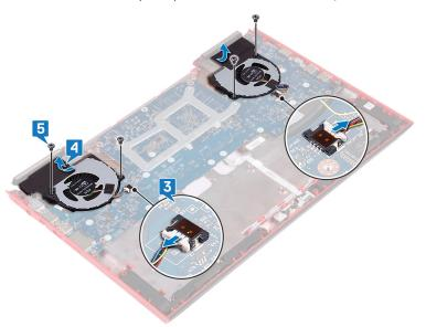
6 Lift the fans off the heat sink.
