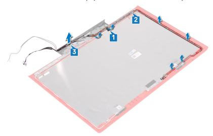
After performing the above steps, we are left with the display back-cover and antenna assembly.
