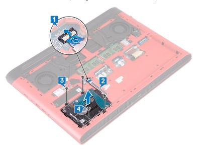
**5** Disconnect the interposer from the hard-drive assembly.
