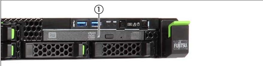
Figure 15: Indicator on the optical drive
