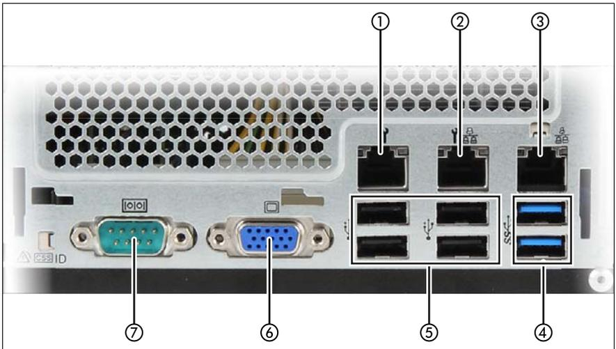
Figure 7: Connector panel on the rear side
