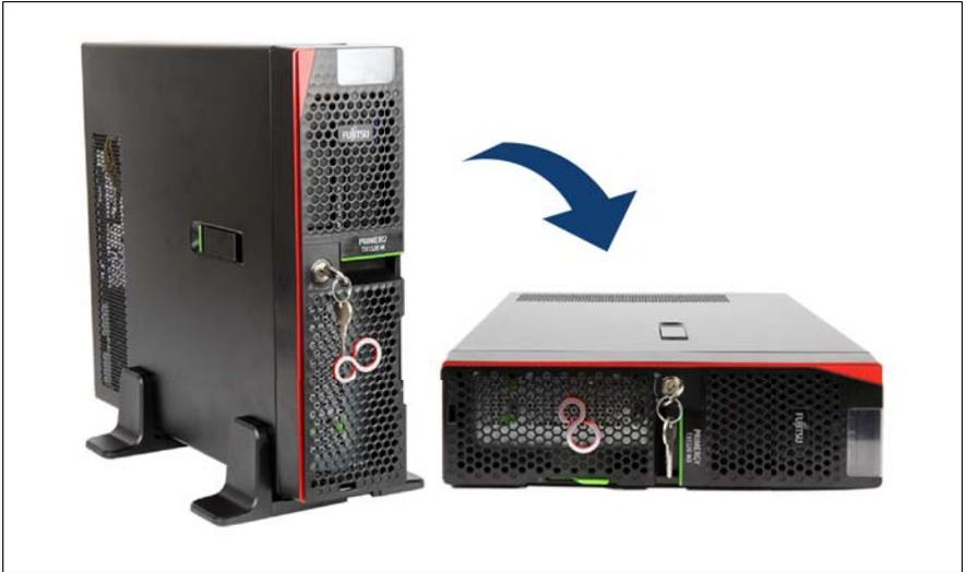
Figure 5: Positioning the server horizontally
