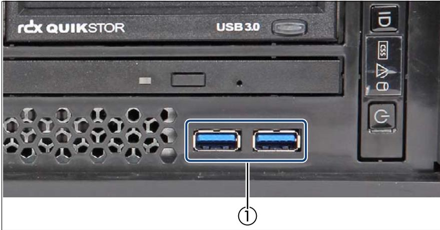
Figure 6: Connectors on the front
