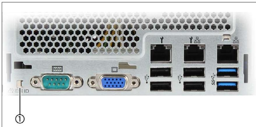
Figure 17: Indicator on the I/O panel: CSS, Global Error and ID indicator
