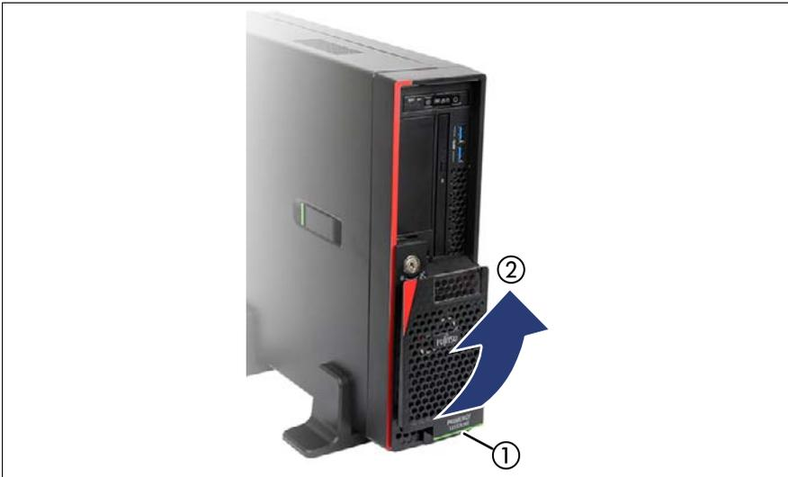
Figure 11: Removing the drive cover from the HDD cover
