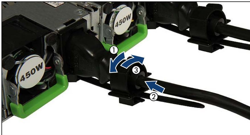
Figure 9: Using cable clamps
