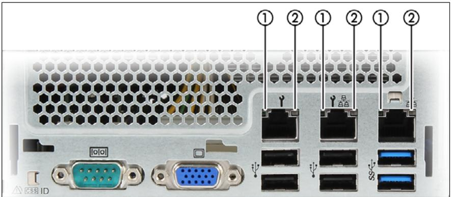
Figure 18: Indicators on the I/O panel: LAN indicators
