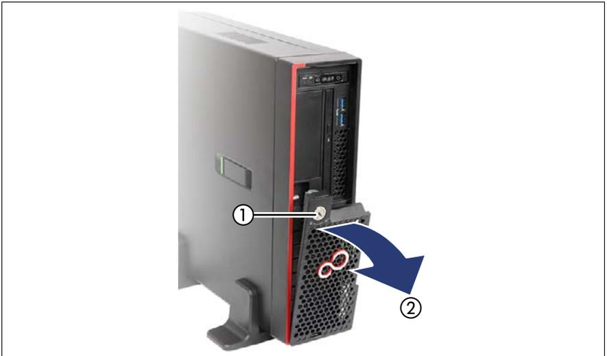
Figure 12: Removing the HDD cover
