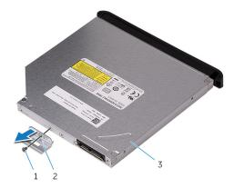
Figure 43. Removing the optical drive
