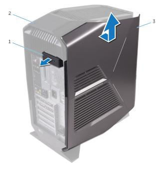
Figure 2. Removing the left-side cover
