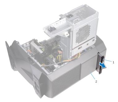
Figure 42. Removing the optical drive
