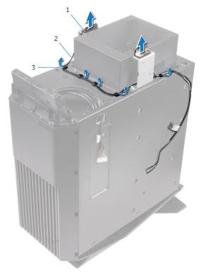
Figure 36. Removing the antenna cables
