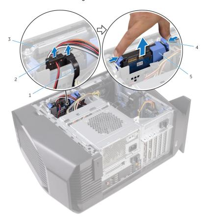
Figure 13. Removing the hard drive
