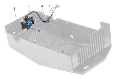
Figure 47. Removing the power-button module
