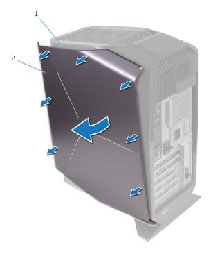
Figure 4. Removing the right-side cover
