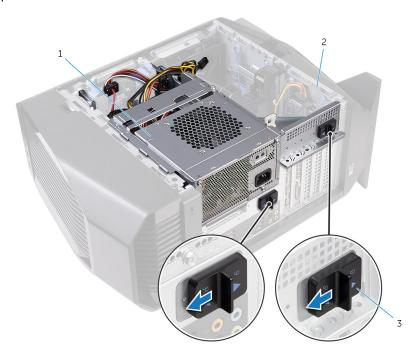
Figure 18. Sliding the power-supply unit cage release latches
