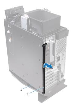
Figure 49. Removing the rear trim cover
