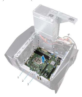
Figure 51. Removing the system board
