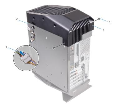
Figure 8. Removing the top cover
