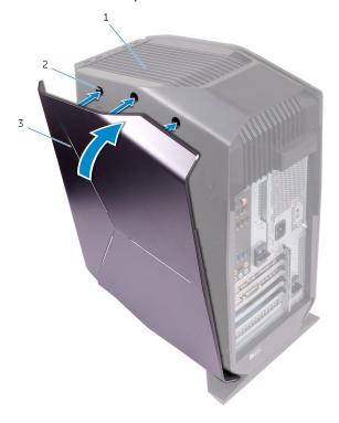
Figure 7. Replacing the right-side cover
