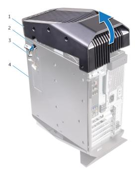
Figure 9. Removing the top cover
