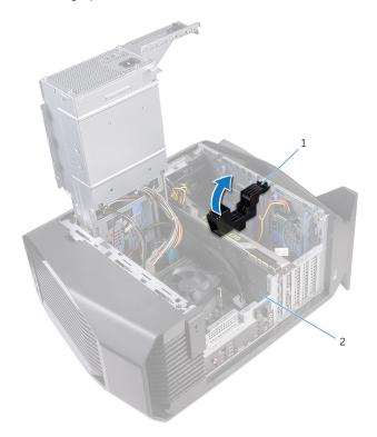
Figure 27. Removing the graphics card
