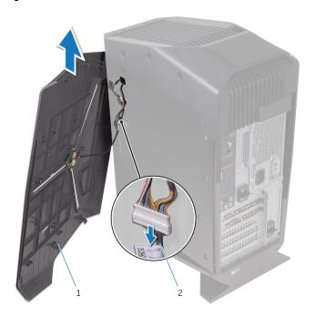
Figure 5. Removing the right-side cover
