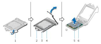
Figure 31. Removing the processor
