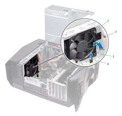
Figure 39. Removing the top-chassis fan
