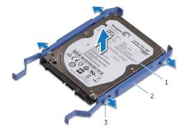
Figure 16. Removing the hard drive from the hard-drive carrier
