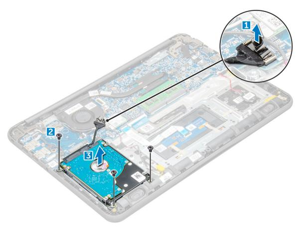
Disconnect the HDD cable interposer.
