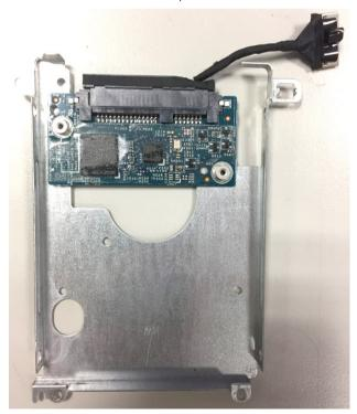
Flip the hard drive bracket, remove the screws (M2.0) and take out the eMM card from the bracket.
