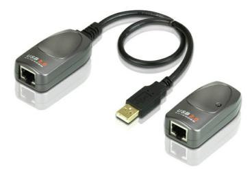
UCE260 can easily send the USB signals via Cat.5/5e/6 cable up to 60 meters (196 ft) at data rate of High Speed (480Mb/s) , Full Speed (12Mb/s) and Low Speed (1.5Mb/s). Without any configuration or software driver, this USB extender allows you to extend your USB device or hub up to 60m from your computer, which overcomes the typical USB cable limitation.
