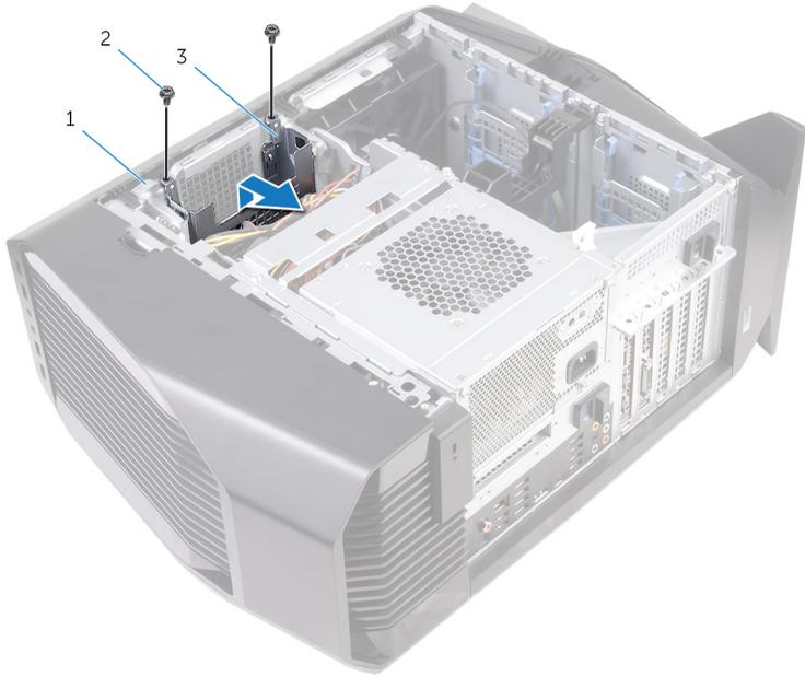
**Figure 17. Removing hard-drive cage**
