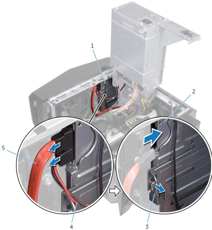
**Figure 41. Disconnecting the power and data cables**
