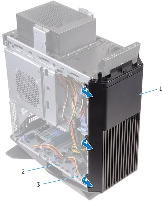
**Figure 45. Removing the front bezel**
