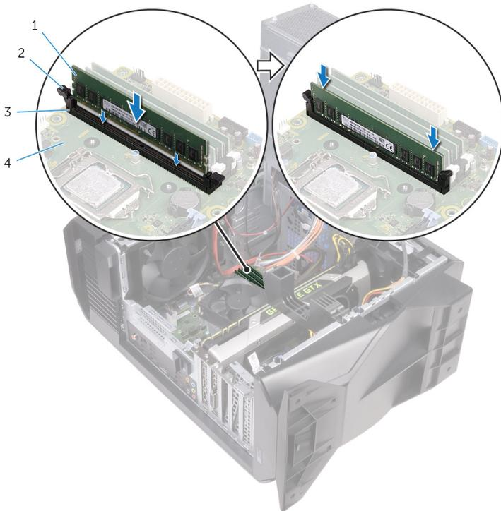
**Figure 26. Replacing the memory module**
