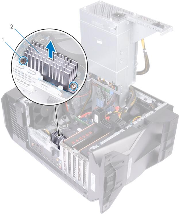
**Figure 29. Removing the VR heat sink**
