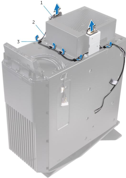
**Figure 36. Removing the antenna cables**
