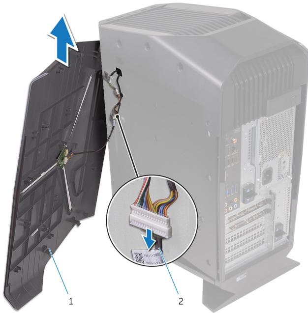
**Figure 5. Removing the right-side cover**
