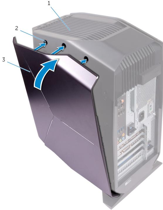
**Figure 7. Replacing the right-side cover**
