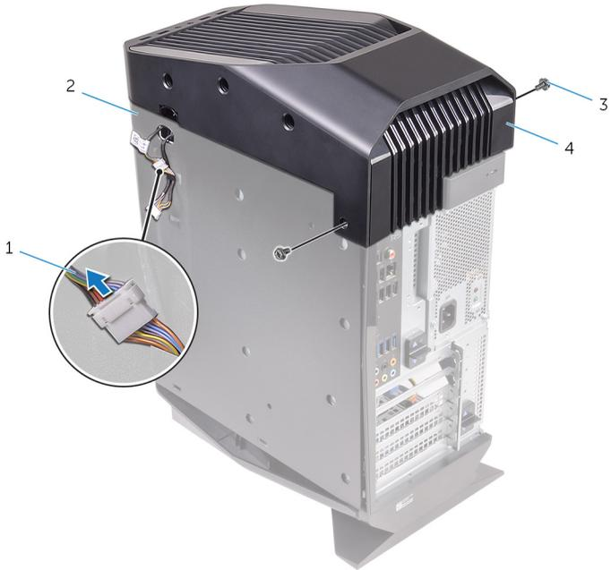
**Figure 8. Removing the top cover**
