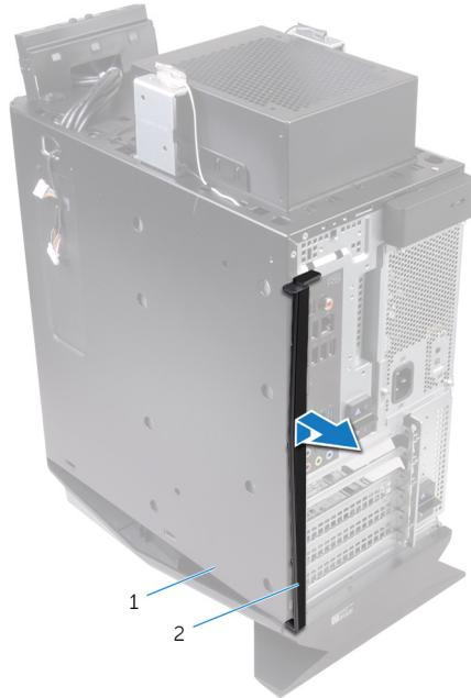
**Figure 49. Removing the rear trim cover**
