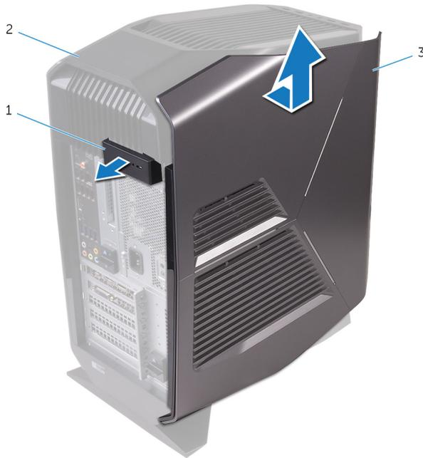
**Figure 2. Removing the left-side cover**
