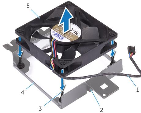
**Figure 40. Removing the top-chassis fan**
