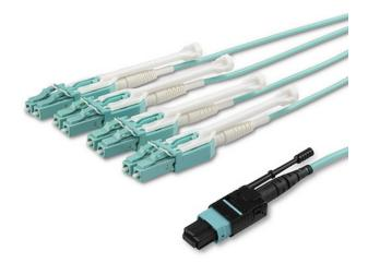
This MPO/MTP to 4x LC breakout cable lets you fan out a single 40Gbps connection from a 40GBase-SR4 QSFP+ transceiver to four 10Gbps LC SFP+ transceivers.
