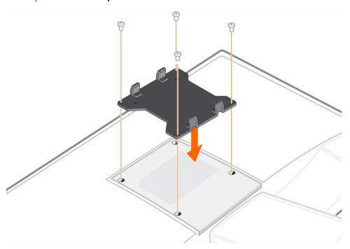
2 Attaching the thin client —Align the thin client over the bracket and gently push the client in place until you hear a click.
