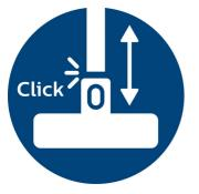
ActiveLock couplings mean nozzles and accessories simply snap into place on the telescopic tube during cleaning.
