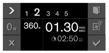
Note: You can set a stabilisation time between two microwave outputs so that the temperature is distributed evenly within the food. To do this, touch the  $O_{\text{W}}$  symbol and set a time using the rotary selector.
