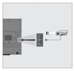
Plug the external hard disk to the USB1 or USB2 USB interface of the television;
