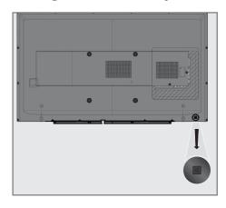
७/I Switches the television on and back into standby mode.
