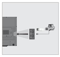
1 Connect the USB1 or USB2 USB interface on the television and the related data output on the external device (external hard disk, digital camera, card reader or MP3 player) with a USB cable;
