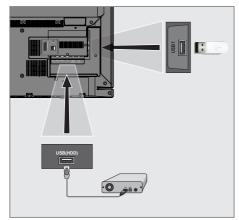
Plug the external hard disk to the USB(HDD) USB interface of the television;
