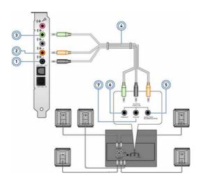
Rear audio connector on the 5 Center/LFE surround out on 1 the speaker computer 2 Center/LFE surround out on Front audio connector on the 6 the computer speaker 3 Front audio connector on 7 Rear audio connector on the the computer speaker 5.1 channel audio cable 4
