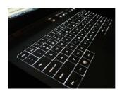
The backlit keyboard on Dell laptops have different lighting states. Press the <Fn> and the right-arrow key to toggle between the various lighting states.
