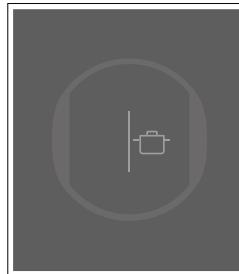
If this symbol appears in the cooking position display, the settings could not be transferred fully. Lift the cookware or move it on the cooking surface. Make the settings for the cooking position again.
