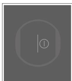
The displayed cooking position has been detected. To select the cooking position, touch the ① symbol.
