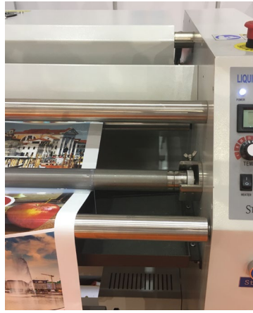
Liquid lamination machine
