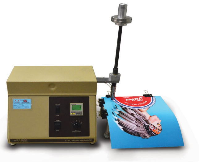
Figure 1 Scratch and abrasion testing are performed using a Taber tester, according to industry-standard test methods. 5
