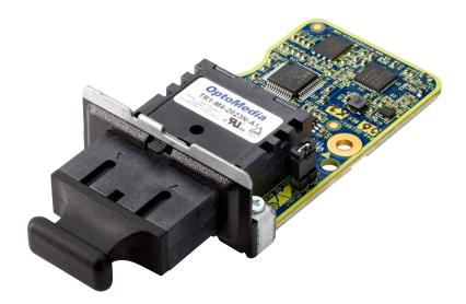
Maximize PC life as your business needs change with the HP Fiber NIC Port Flex IO that offers superb transfer rates, reliability, and security versus standard Ethernet connections.
