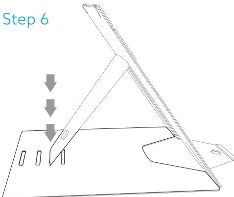
Insert the support in the slot of your desired height
