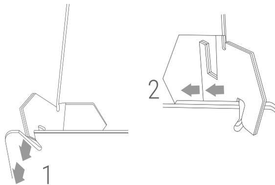
Move the tablet hook onto the slot (1) and then move the hook around the middle plate (2) until the hook is right-angled with the middle plate
