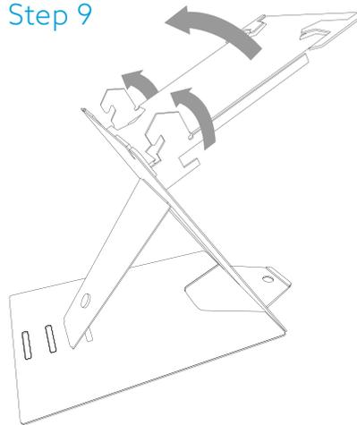
And turn both tablet support at the same time (use both hands). Make sure you turn the tablet support until the hook is in front of the tablet slot
