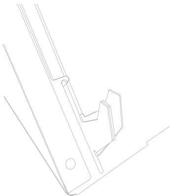
The top plate rest on the middle plate and the laptop supports are in the laptop slot. The laptop stand is now ready to use!
