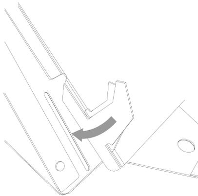
Lower the top plate and make sure that both laptop supports go into the laptop slot
