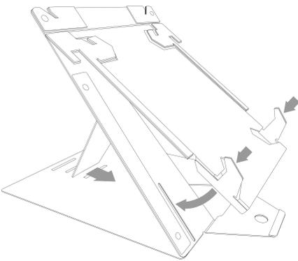
Turn both laptop supports (2). Make sure that both laptop supports are right angles to the top plate
