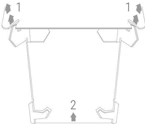
Make sure that the hooks of the tablet supports go into the tablet slots, while (1) lifting the top plate until it is vertical
