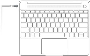
Your MateBook X is pre-installed with an irremovable, rechargeable battery. You can charge your MateBook X with the adapter and USB-C charging cable that comes with it. The battery is sufficiently charged when the charging indicator stays steady white.
