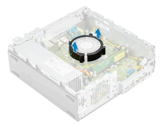
b Loosen the 4 captive screws that secure the heat sink [1] and lift it away from the system [2].
