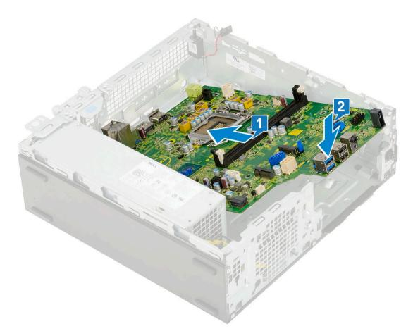
3 Replace the single (#6-32) screw, single (M3x5) screw and 5 screws that secure the system board to the system [1, 2, 3].
