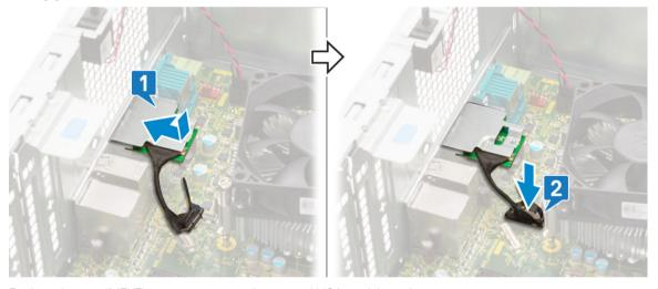
3 Replace the two (M3X3) screws to secure the optional VGA module to the system.
