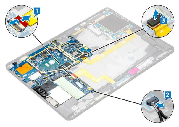
Un route the antenna cables from the routing clips [1,2,3].
