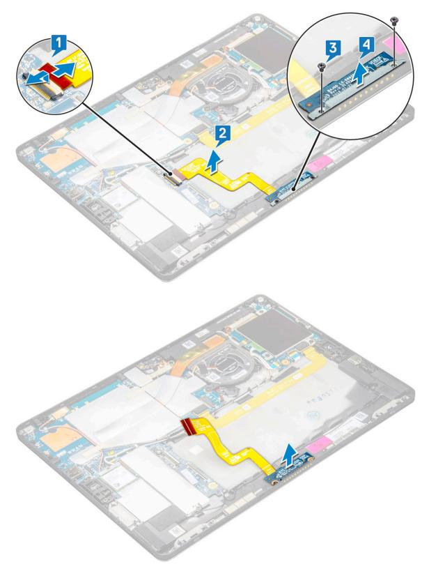
Lift the docking board after releasing the cable from the adhesive.
