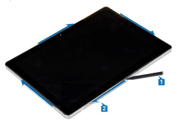
7 Flip the display panel on a plane surface with the LCD panel upwards.
