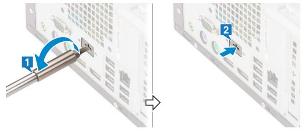
2 Insert the VGA module into its slot from the inside of your computer [1] and connect the VGA cable to the connector on the system board [2].
