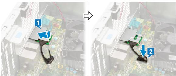
3 Replace the two (M3X3) screws to secure the optional VGA module to the system.
