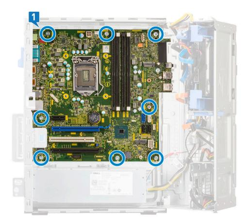
b Slide and lift the system board away from the computer [1, 2].
