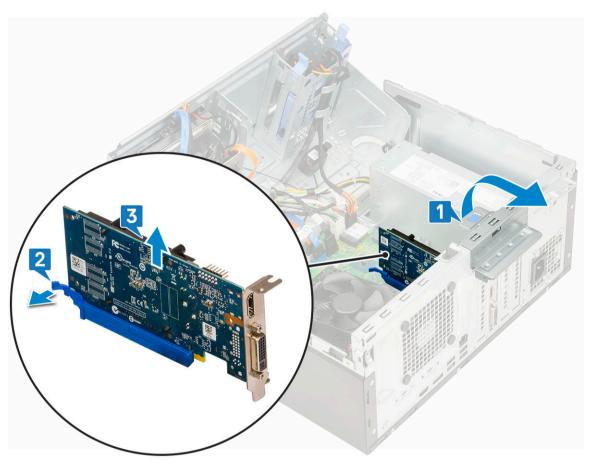
5 Repeat the steps to remove any additional PCIe expansion card.
