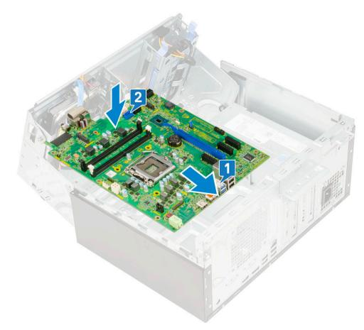
3 Replace the screws to secure the system board to the computer [1].
