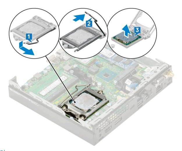
(i) NOTE: After removing the processor, place it in an antistatic container for reuse, return, or temporary storage. Do not touch the bottom of the processor to avoid damage to the processor contacts. Touch only the side edges of the processor.
