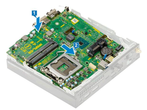
c Replace the two (M3x4) screws [1] and three (6-32x5.4) screws [2] to secure the system board to the system.
