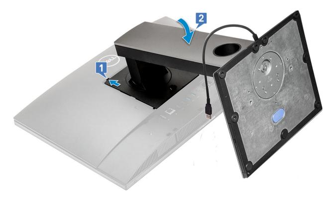
3 Connect the optical drive cable to the USB slot on the back cover.
