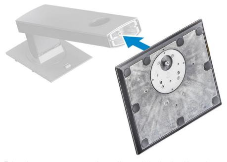
3 Tighten the captive screw to secure the stand base to the height adjustable stand.
