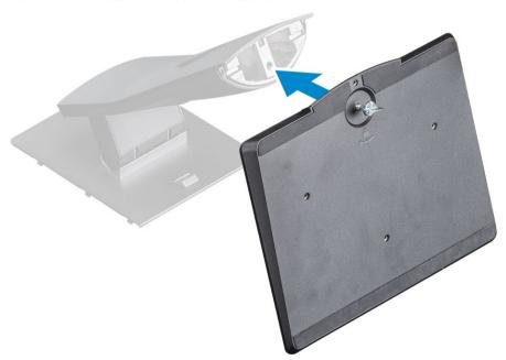
3 Tighten the captive screw to secure the stand base to the basic stand.
