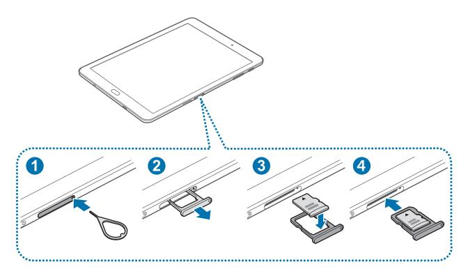
1 Insert the ejection pin into the hole on the memory card tray to loosen the tray.
