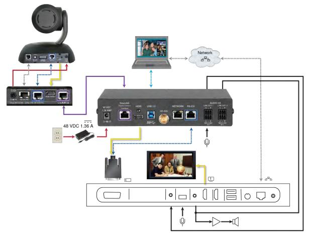
This diagram shows the camera and OneLINK HDMI extension connected to the codec and separately providing an IP video stream. It depicts the required Polycom fan-out cable and the signal types it carries. The OneLINK HDMI extension also provides IR forwarding.
