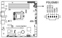
P10S-M WS Series Power supply SMBus connector
