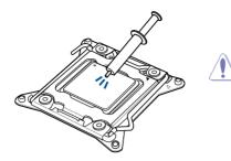
Apply the Thermal Interface Material to the CPU heatsink and CPU before you install the heatsink and fan, if necessary.
