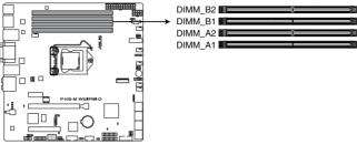
P10S-M WS Series 288-pin DDR4 DIMM sockets
