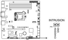
P10S-M WS Series Chassis Intrusion connector
