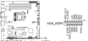
P10S-M WS Series Internal VGA connector
