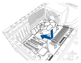
Place eight (8) screws into the holes indicated by circles to secure the motherboard to the chassis.
