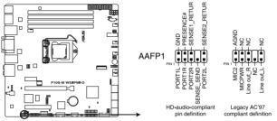
P10S-M WS Series Analog front panel connector
