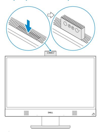
1 NOTE: Extend the camera while using any camera function so that the camera is not blocked.
