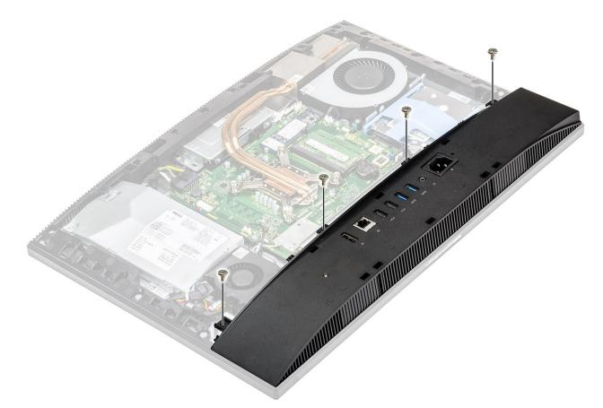
4 Pry and lift the base cover off the middle frame.
