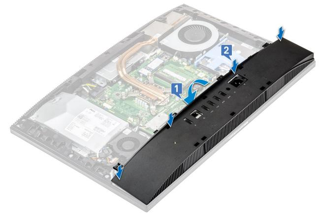
3 Replace the four screws (M3) that secure the base cover to the display assembly base.
