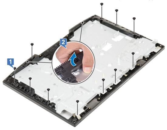
5 Lift the middle frame off the display assembly base [1].
