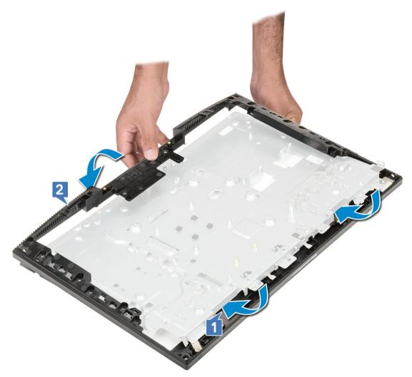
2 Replace the 11 screws (M3x5) that secure the middle frame to the display assembly base [2].
