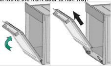
Remove the front door by pulling it upwards to release it from the right and left hinges.
