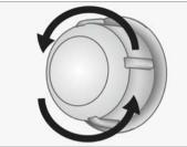
3. If your oven lamp is of type (A) shown in the figure below, remove it by rotating as shown and replace it. If it is of type (B), pull and remove it as shown in the figure and replace it.
