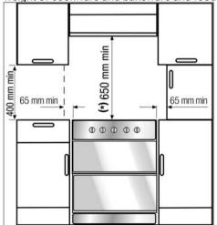
It can be used with cabinets on either side but in order to have a minimum distance of 400 mm above hotplate level allow a side clearance of 65mm
