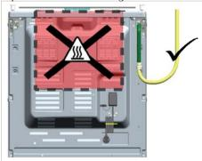
If the gas hose outlet and the natural gas valve do not face the same side, make sure that the hose does not pass through the hot area when connecting it.
