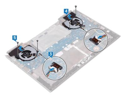
6 Lift the left and right fans off the heat sink.
