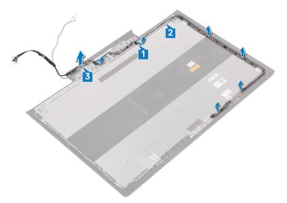
4 After performing the above steps you are left with the display back-cover and antenna assembly.
