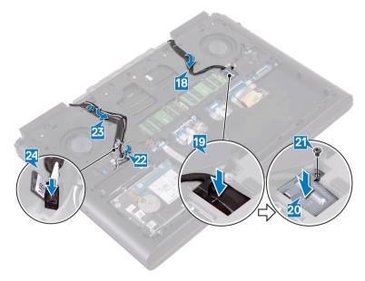
25 Adhere the tapes that secure the display cable, camera, and antenna cables to the computer base.
