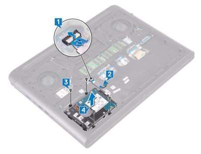
Disconnect the interposer from the hard-drive assembly.
