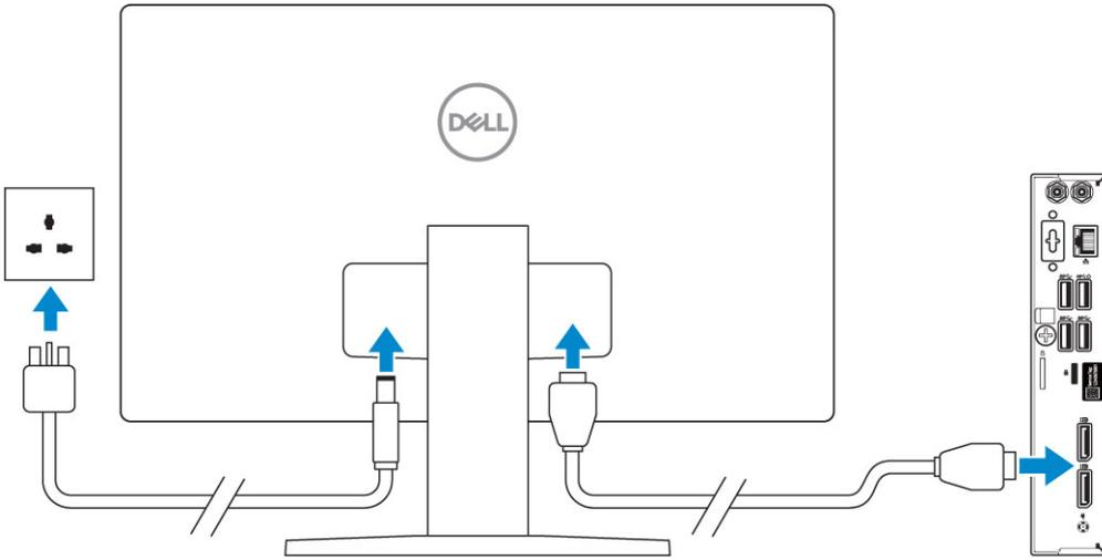
**NOTE:** If you ordered your computer with a discrete graphics card, the HDMI and the display ports on the back panel of your computer are covered. Connect the display to the discrete graphics card.
