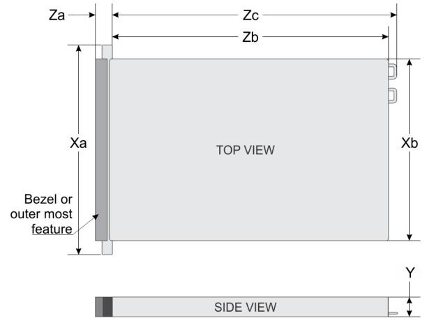
Figure 1. Dimensions of the PowerEdge R7415 system
