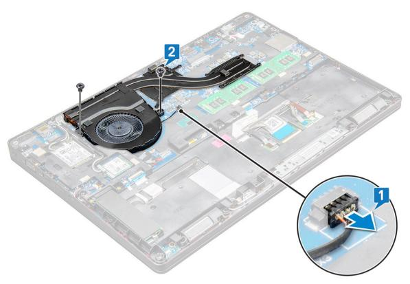
b Remove the screws M2x3 (6) that secures the heat sink on the system board [1].
