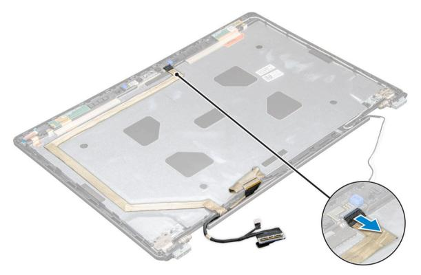
4 Peel off the eDP cable from the adhesive to remove it from the display.
