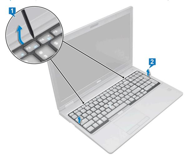
NOTE: Use a plastic scribe to pry the keyboard lattice from the pry points and move around the lattice for removal.
