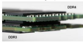
Figure 2. Thickness difference
